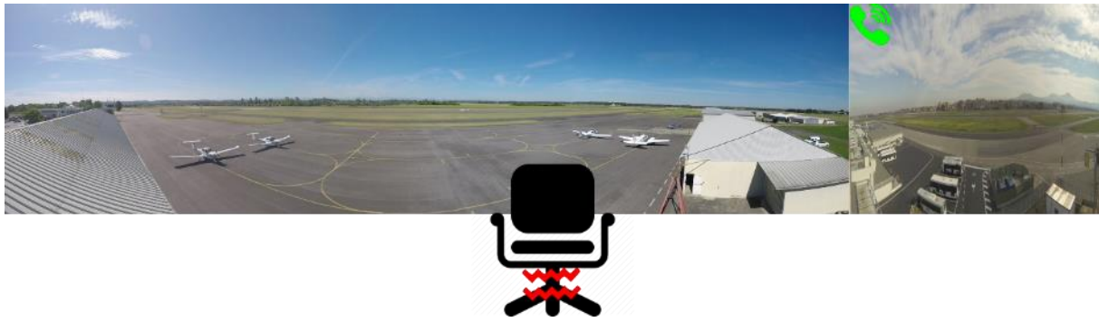
Figure 9. Vibration of the seat of the chair to indicate to the ATCO, that the call is coming from a secondary airport.
