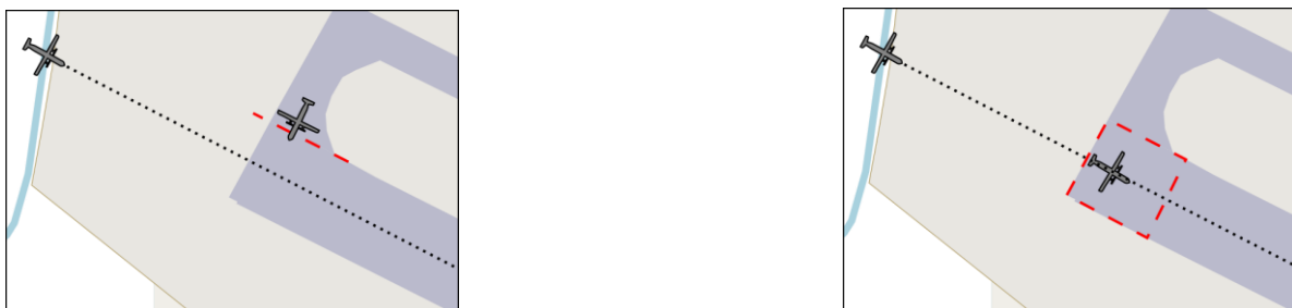
Figure 10. Left: Runway incursion due to a holding point crossing w/o authorization. Right: Runway incursion due to an aircraft lined up. Center: Vibration alarming the ATCO that a runway incursion has been detected.
